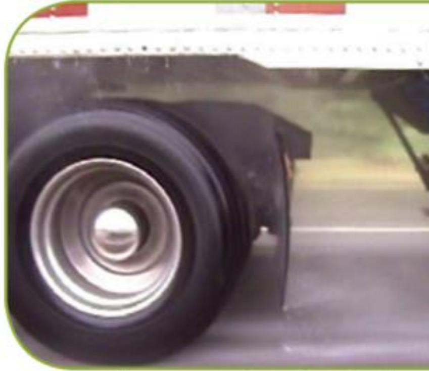
The solid flap blocks air flow coming around the tires and creates turbulence that picks up standing water and jettisons it in big clouds of vapor
